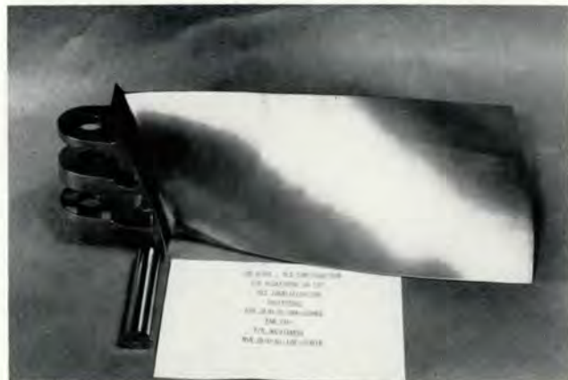
Good News! These original TF34 engine fan blades used to be discarded after 3,000 hours. Now they can be reworked and reused.
