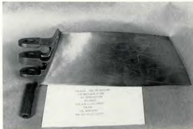
Bad News! These new blades are not Murphy proof and can be erroneously intermixed with the old fan blades in a rotor assembly.
